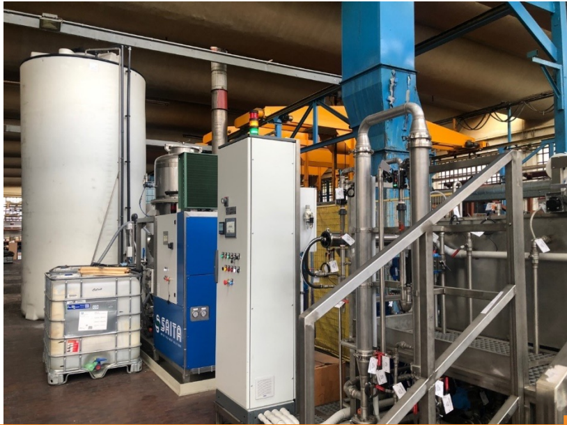
Figure 1 – Ultrafiltration and distillation system operating at CleanAir Europe S.r.l.
